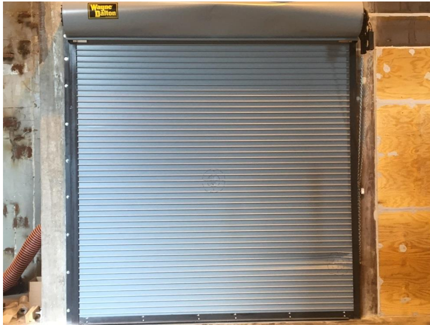
Photo No. 1 Test Specimen #1 after Impact Testing with an Exterior Installation
